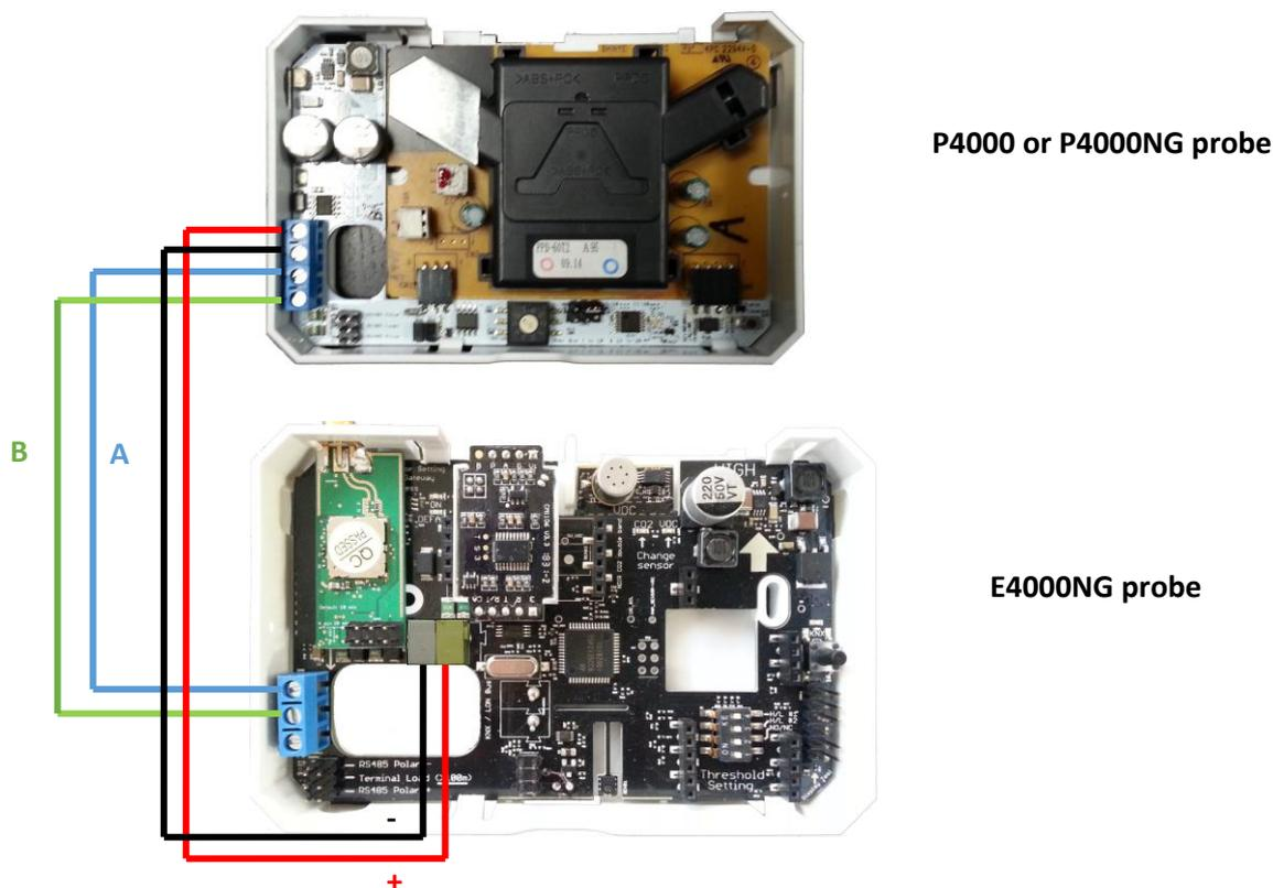
A non-twisted cable can be used if the auxiliary probe is close (<2m). Do not use jumpers if the distance is <100m.
