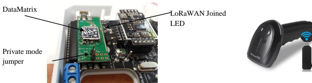
At startup, the radio module will automatically be recognized by the LoRaWAN network. When the radio module is connected to the LoRaWAN network, the green LED of the radio module is On. Be careful, recording on an operated network may require several radio transmission cycles.
