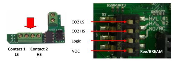
The two dry contacts are activated according to CO2, VOC or relative Humidity thresholds depending of the 4 deep switch configurations (see installation manual for details):
