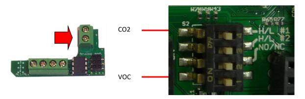
Only the #4 deep switch used for the dry contacts allows a setting of High or Low threshold of CO2 for the 1-10V output.
